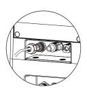
3. Plug the other end of the CAN communication cable to the CAN connector on BMS. Tighten the screw cap at the end of the cable.
