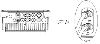
2. Connect the negative cable (-) (B)to the port on the right and the positive cable (+) (A) to the one on the left shown as in the figure.
