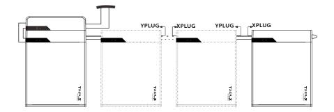
2. After all the battery modules were correctly connected, plug the short-circuit plug (F) at YPLUG ( $\mathbf{V}'$ ) of last battery module to make a complete circuit.
