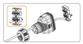
Figure 8-57 Installing RJ45 terminal to the cable fixture
