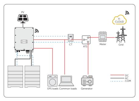
Figure 14-1 ATS control wiring diagram
