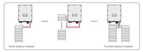
Figure 8-32 Inverter with split battery modules
