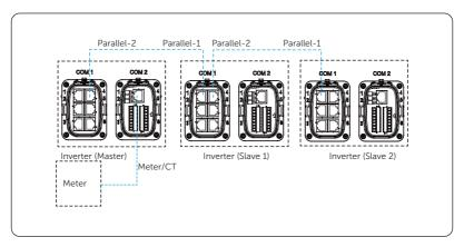
Figure 14-19 Communication wiring without X3-PBOX-300kW
