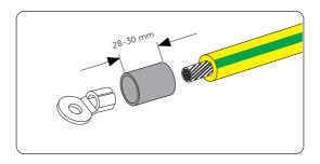
Figure 8-3 Installing the tubing and OT teriminal
