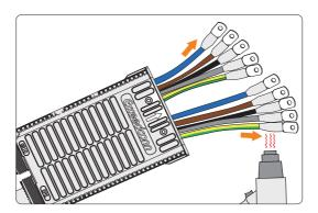
Figure 8-17 Shrinking the tubings
