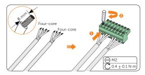
Figure 8-77 Connecting to 8-pin terminal block
