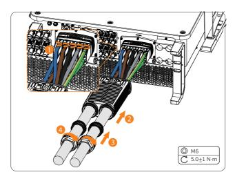
Figure 8-19 Connecting the EPS cable
