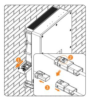
Figure 11-3 Releasing the fan waterproof connectors
