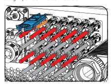
Figure 12-2 Releasing the PV connector
