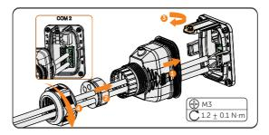
Figure 8-78 Connecting to the inverter
