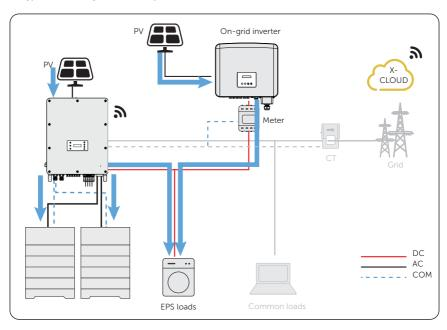
Figure 14-12 Power flowing when grid off
