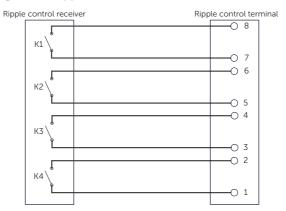
Figure 8-70 Connection diagram for ripple control
