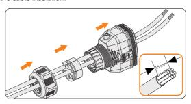
Figure 8-47 Threading the cables and striping the insulation
