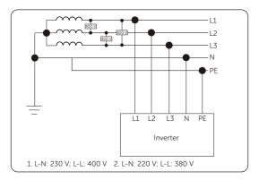
Figure 2-4 Supported power grid-TN-C-S
