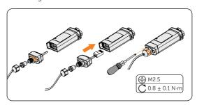
Figure 8-84 Assembling the LAN dongle
