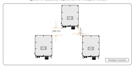
Figure 5-6 Clearance requirement for multiple inverters
