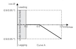
» \*) If the inverter Pmax ≤ 4.6kW, the Power Factor is 0.95 at 1.0 power; if the inverter Pmax > 4.6kW, the Power Factor is 0.90 at 1.0 power.
