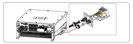
Figure 14-9 Connecting to EV-Charger
