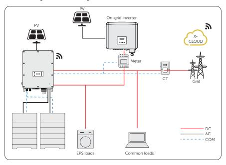
Figure 14-10 Micro-grid wiring connection
