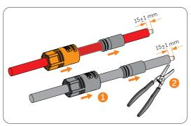
Figure 8-36 Stripping the battery power cable
