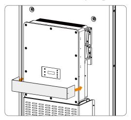
Figure 7-21 Putting the screen cover on the inverter
