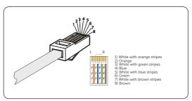
Figure 8-56 Crimping the communication cable
