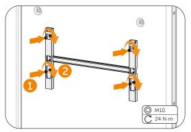
Figure 7-15 Securing the mounting bracket
