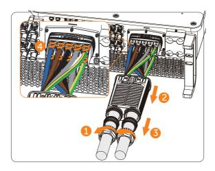
Figure 12-5 Removing AC terminals
