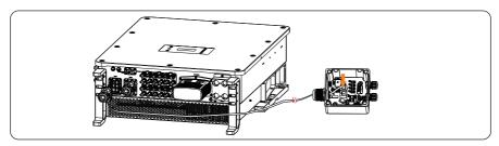
Figure 14-6 Connecting to Adapter Box
