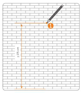
Figure 7-5 Marking the first hole
