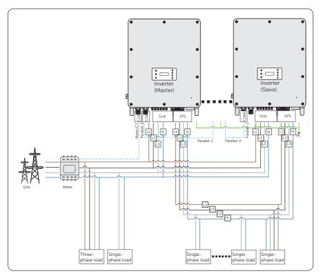
Figure 14-15 Without X3-PBOX-300kW system wiring diagram
