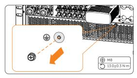
Figure 8-6 Uninstalling the screw
