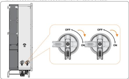
• Turn off the DC switch: rotate the DC switch from ON state to OFF state.
