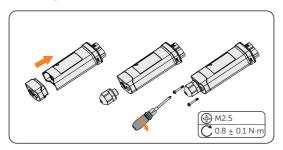
Figure 8-81 Assembling the dongle
