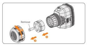
Figure 8-65 Disassembling the connector
