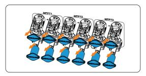
Figure 8-28 Connecting the PV cable
