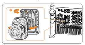
Figure 8-64 Disassembling the COM 2 terminal
