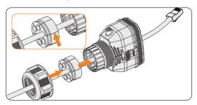
Figure 8-66 Threading the cable with RJ45 terminal
