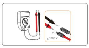
Figure 8-27 Measuring the voltage of PV connectors
