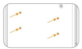
Figure 7-14 Confirming the position of the mounting bracket
