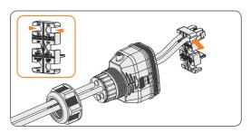
Figure 8-49 Installing the cable to the cable fixture
