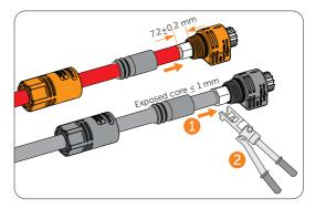
Figure 8-37 Crimping the terminal
