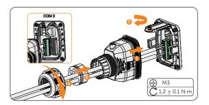
Figure 8-75 Connecting to the inverter
