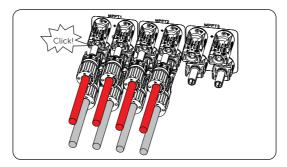
Figure 8-29 Connecting assembled PV cables to the inverter
