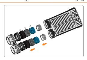
Figure 8-13 Disassembling the swivel nuts
