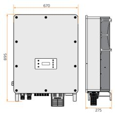
Figure 7-3 Dimensions 1 (Unit: mm)
