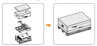
Figure 12-9 Packing the inverter
