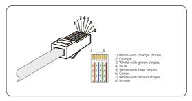
Figure 8-48 Crimping the communication cable
