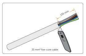
Figure 8-8 Striping the Grid cable
