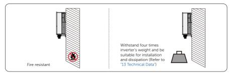
Figure 5-3 Installation carrier requirement
