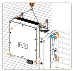
Figure 12-8 Lifting down the inverter
