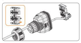
Figure 8-59 Installing RJ45 terminal to the cable fixture
