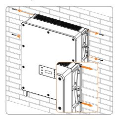
Figure 12-6 Unscrewing screws on the inverter
