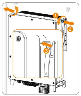
Figure 7-19 Removing the eye bolts
