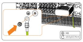
Figure 8-7 Securing the PE cable
