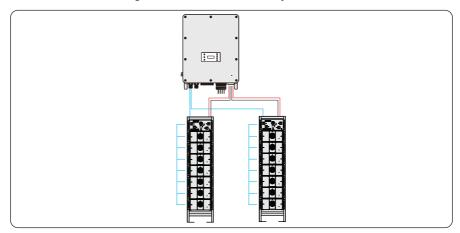
Figure 8-34 Inverter with battery bracket
