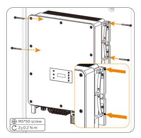
Figure 7-20 Securing the inverter
