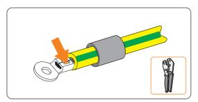
Figure 8-4 Crimping the cable
