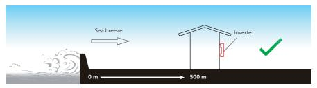
Figure 5-1 Recommended installation position
