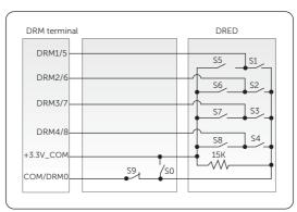
Figure 8-58 DRED connection diagram
