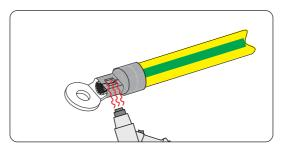
Figure 8-5 shrinking the tubing
