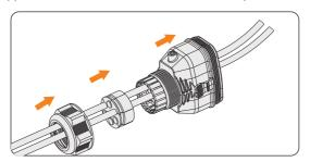
Figure 8-73 Threading the cables
