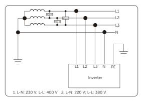
Figure 2-2 Supported power grid-TT
