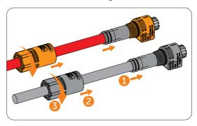
Figure 8-38 Tightening the battery connector
