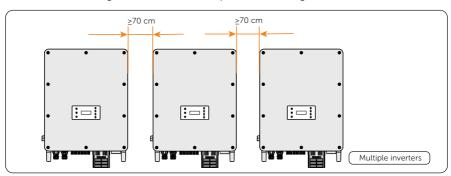
Figure 5-5 Clearance requirement for multiple inverters
