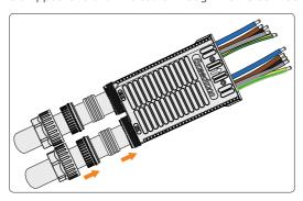
Figure 8-14 Threading cables through the AC connector
