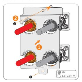
Figure 8-42 Installing the battery proctective cover
