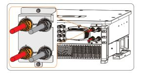
Figure 8-43 Well connected battery cables
