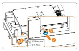
Figure 7-16 Installing the eye bolts
