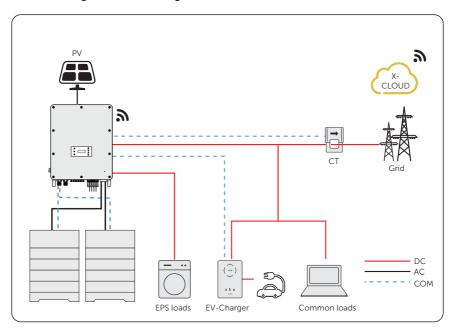
Figure 14-7 EV-Charger wiring diagram
