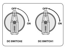
Figure 12-1 Turning off the DC switch
