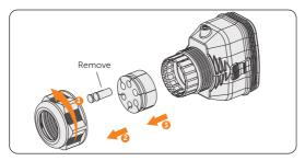
Figure 8-72 Disassembling the connector
