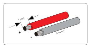
Figure 8-22 Striping the PV cable
