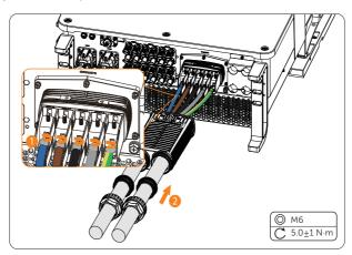
Figure 8-18 Connecting the Grid cable
