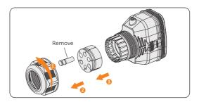
Figure 8-45 Disassembling the connector
