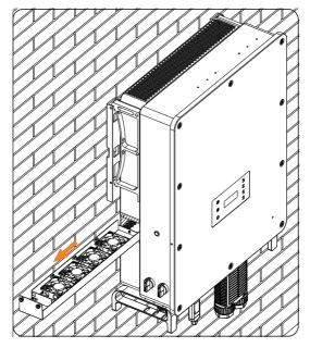
Figure 11-4 Pulling put the whole fan bracket
