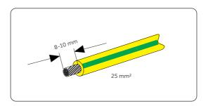
Figure 8-2 Striping the PE cable
