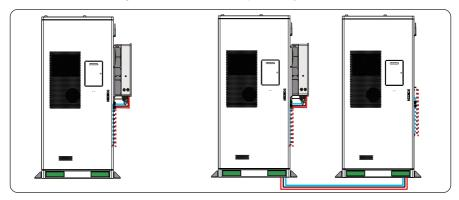
Figure 8-33 Inverter with battery cabinet(s)
