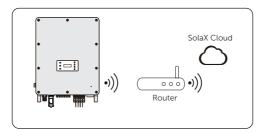
Figure 8-79 Wi-Fi mode connection diagram
