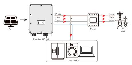
Figure 2-16 Zero export control with Phase Unbalance enabled
