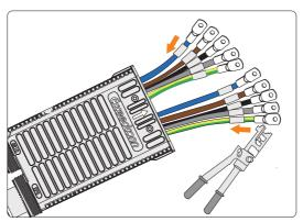
Figure 8-16 Crimping AC terminals
