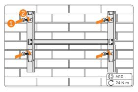
Figure 7-8 Securing the mounting bracket
