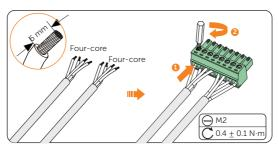
Figure 8-74 Connecting to 8-pin terminal block
