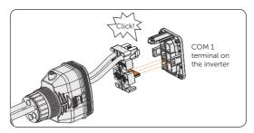
Figure 8-50 Inserting the connector to COM 1
