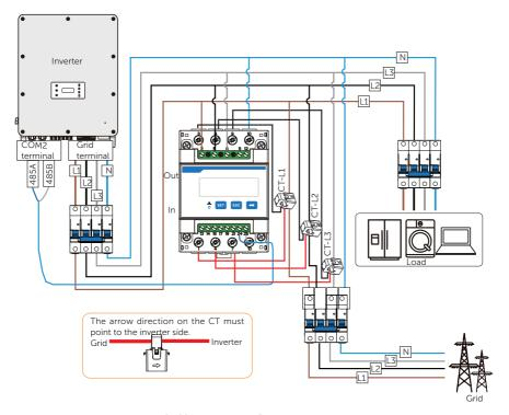
Figure 8-62 Meter with CT connection diagram
