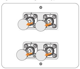
Figure 8-40 Removing battery caps
