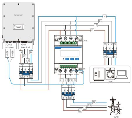
Figure 8-60 Meter connection diagram 1
