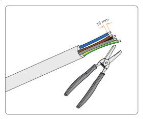
Figure 8-11 Stripping cables
