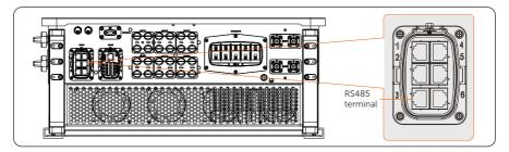
Figure 14-8 Connection terminal for EV-Charger
