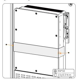
Figure 7-22 Securing the cover with the inverter
