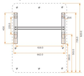
Figure 7-4 Dimensions 2 (Unit: mm)
