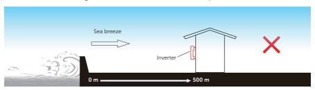
Figure 5-2 Incorrect installation position
