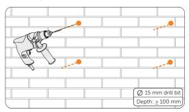
Figure 7-7 Drilling holes
