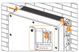
Figure 7-12 Removing the eye bolts
