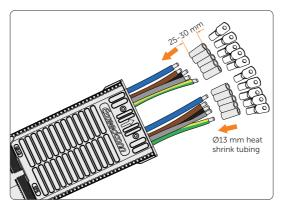
Figure 8-15 Assembling tubings and AC terminals
