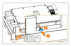
Figure 7-9 Installing the eye bolts
