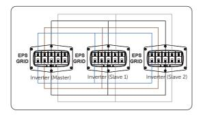
Figure 14-17 Power cable wiring without X3-PBOX-300kW
