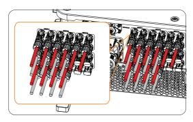
Figure 8-31 Well connected PV cables and dustproof buckles
