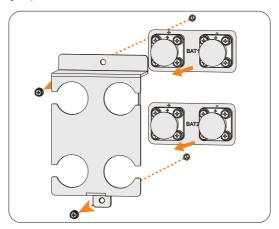
Figure 8-39 Removing the battery protective cover
