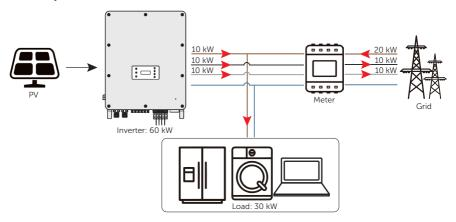
Figure 2-15 Zero export control with Phase Unbalance disabled
