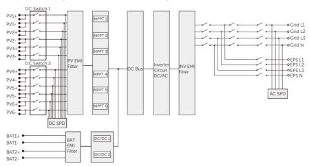
Figure 2-5 Circuit Diagram for X3-AELIO series inverter
