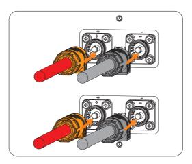
Figure 8-41 Connecting assembled battery cables
