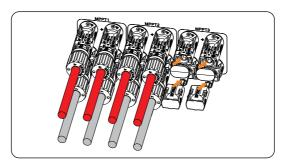
Figure 8-30 Installing PV dustproof buckles
