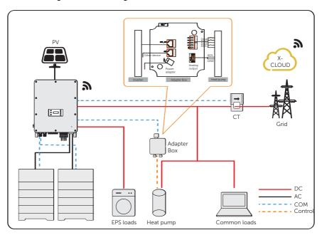
Figure 14-4 Adapter Box wiring diagram
