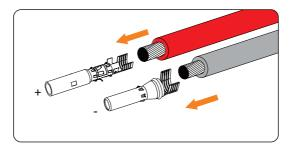
Figure 8-23 Inserting the PV pin contact
