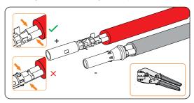
Figure 8-24 Crimping the terminal
