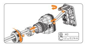
Figure 8-51 Securing the connector
