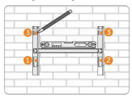
Figure 7-6 Marking the rest holes
