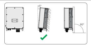
Figure 7-1 Correct installtion
