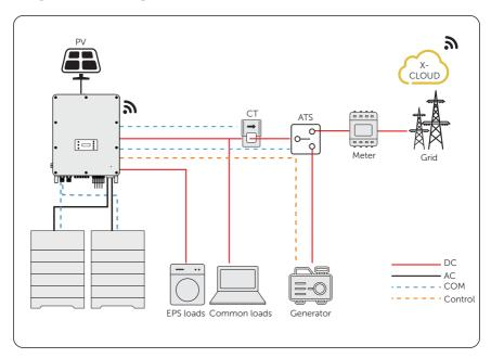
Figure 14-2 Dry contact wiring diagram
