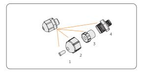
Figure 8-83 Disassembling the waterproof connector
