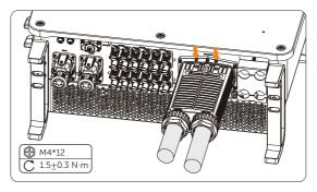
Figure 8-20 Securing the AC connector on the inverter
