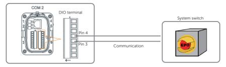
Figure 8-76 System switch connection diagram
