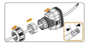
Figure 8-55 Threading the cables and striping the insulation
