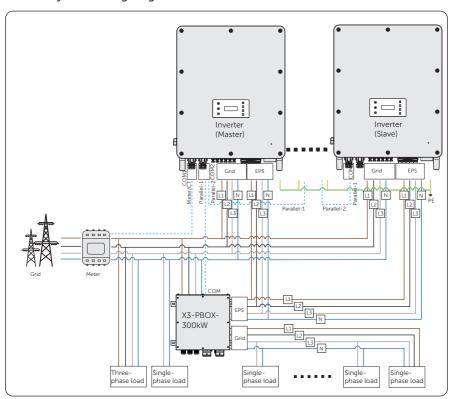
Figure 14-14 With X3-PBOX-300kW system wiring diagram
