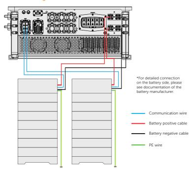
Figure 8-52 BMS connection diagram
