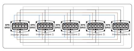
Figure 14-16 Power cable wiring with X3-PBOX-300kW
