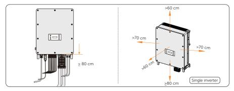
Figure 5-4 Clearance requirement for single inverter
