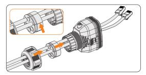
Figure 8-46 Threading the cables with RJ45 terminal
