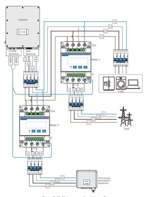
Figure 8-61 Meter connection diagram 2
