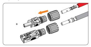
Figure 8-25 Threading the PV cable
