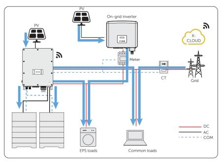
Figure 14-11 Power flowing when grid on and PV sufficient
