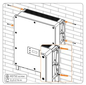
Figure 7-13 Securing the inverter
