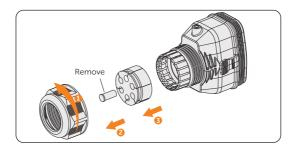
Figure 8-54 Disassembling the connector
