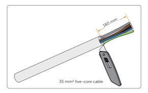
Figure 8-9 Striping the EPS cable
