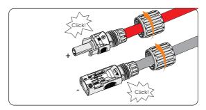
Figure 8-26 Securing the PV cable
