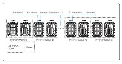
Figure 14-18 Communication wiring with X3-PBOX-300kW
